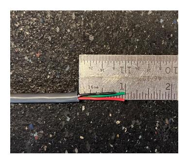
Spread the individual conductors into a fork, as pictured:
