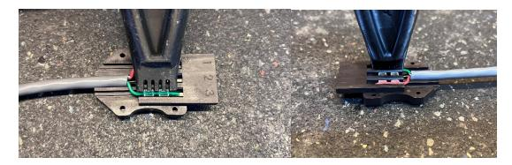
Next, screw the Top onto the Bottom using the supplied screws. Tighten until the top is fully seated on the bottom, there should be no gaps along the seams.
