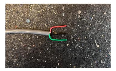
Next, the wires will need to be pushed into the contact clips. This can be done with the push in tool. Pushing the wires into the contacts can also be done with a small flat head screwdriver. It is best to push the wire in evenly and fully!
