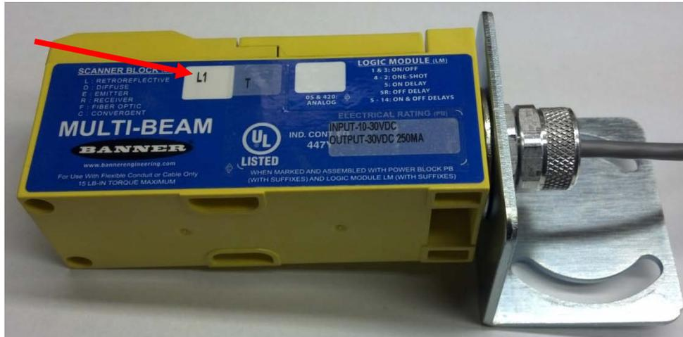
With your track powered and power to your sensors remove the white protective dust cap using a flat head screw driver.
