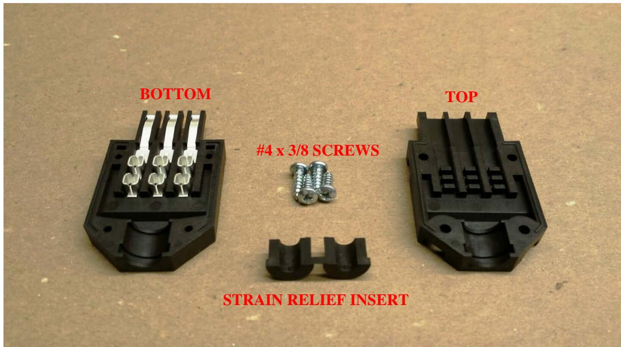
To install the connectors first prepare the wire by stripping approximately 1 inch of the outside jacket off. Also strip approximately 1/16 of an inch of each individual conductor.
